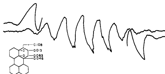
Fig. 3.—Calculated spin densities and observed spectrum of perylene negative ion.
